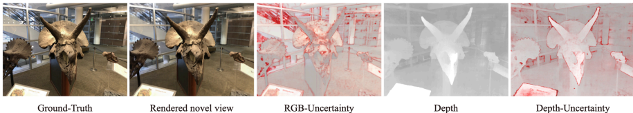
Figure 1. Illustration of the results obtained by Stochastic Neural Radiance Fields (S-NeRF). Our method is a probabilistic generalization of the original NeRF, which is able to not only address tasks such as novel-view generation (Rendered novel view) or depth-map estimation (Depth), but also quantify the uncertainty (red color) associated with the model outputs. This is specially important in domains such as robotics, where this information is necessary to evaluate the risk associated with decisions based on the model estimations.
